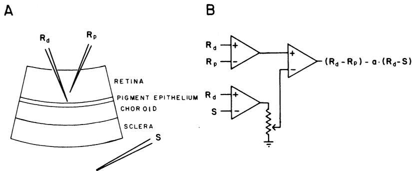
Fig. 6. Arrangement used in recording the mass receptor response. (A) Distal ( $R_d$ ) and proximal ( $R_p$ ) intraretinal electrodes were placed on opposite sides of the receptor layer in the retina. (B) The corrected receptor response was obtained by subtracting a fraction ( $a$ ) of the  $c$ -wave response ( $R_d - S$ ) from the receptor response ( $R_d - R_p$ ).
